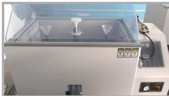
5. Salt Spray Testing
